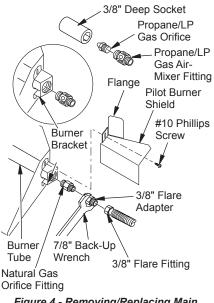
Figure 4 - Removing/Replacing Main Burner Orifice
